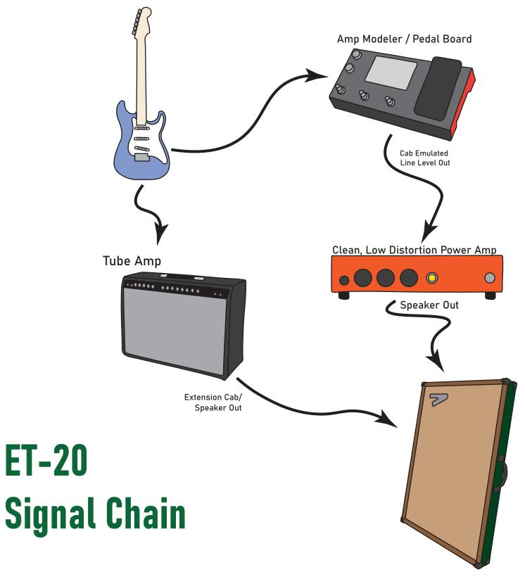
The Eminent Technology Model Twenty is a passive, full range, flat response guitar cabinet. The contour switches on the rear of the Model Twenty give multiple ways to narrow the frequency bandwidth to that of a more traditional guitar speaker. This allows the Model Twenty to be used with clean amplifiers designed to power traditional cabinets. When being used with amp modelers, the full range response of the Model Twenty affords the user accurate reproduction of any cabinet simulation.
