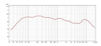
With all of it's switches in the down position, the Model Twenty operates in full range, flat response mode. This configuration is best suited for modelers or any signal paths utilizing cabinet simulation. It is also practical for use with acoustic guitar, keyboard, vocals, or other full range instruments.
